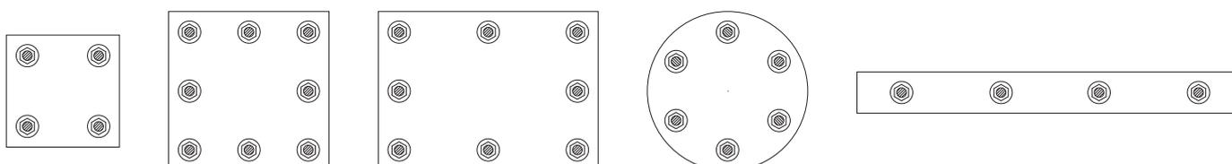
While arranging the anchor bolts, the minimum values as described in table below must be followed. Attention has to be paid to punching resistance under the stud while calculating the thickness of the base structure and reinforcement.
