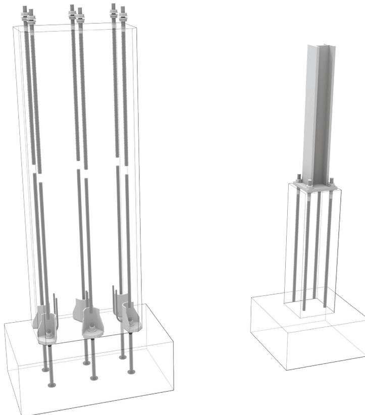
To increase the load-carrying capacity, anchors are assembled in a group. Moreover, this allows for a moment-resisting connection. For tension and shear load, the mechanical behavior is mainly influenced by
