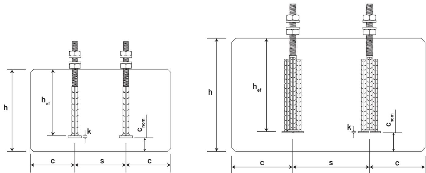
**Table 3. Positioning of SKP -L Type High Capacity Anchor Bolt**
