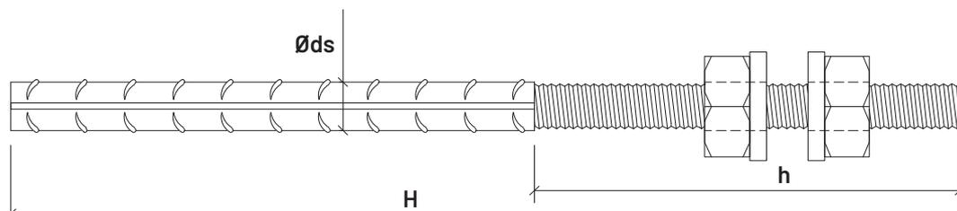
Table 6. SKP - L Type High Capacity Anchor Bolt
