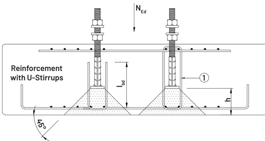
Table 27. Concrete Edge Reinforcement for NKP - L Type
