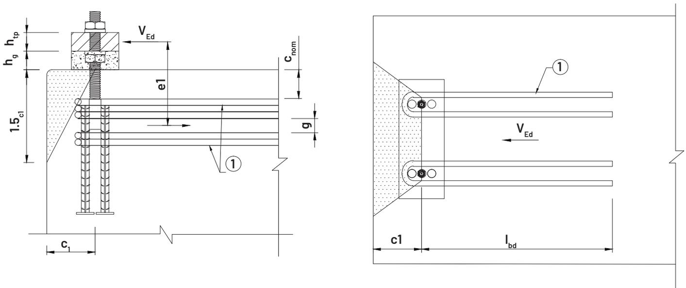
Table 26. Concrete Edge Reinforcement for SKP - L Type High Capacity Anchor Bolt
