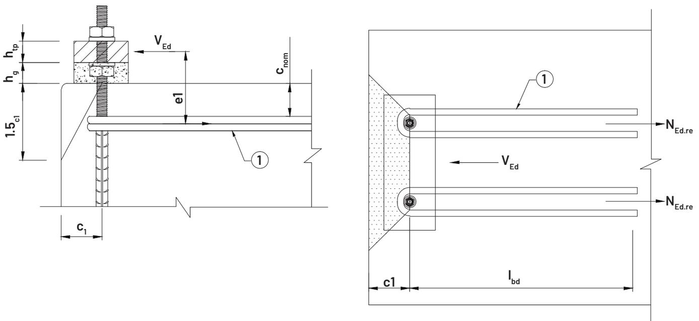
Table 25. Concrete Edge Reinforcement for NKP - L Type
