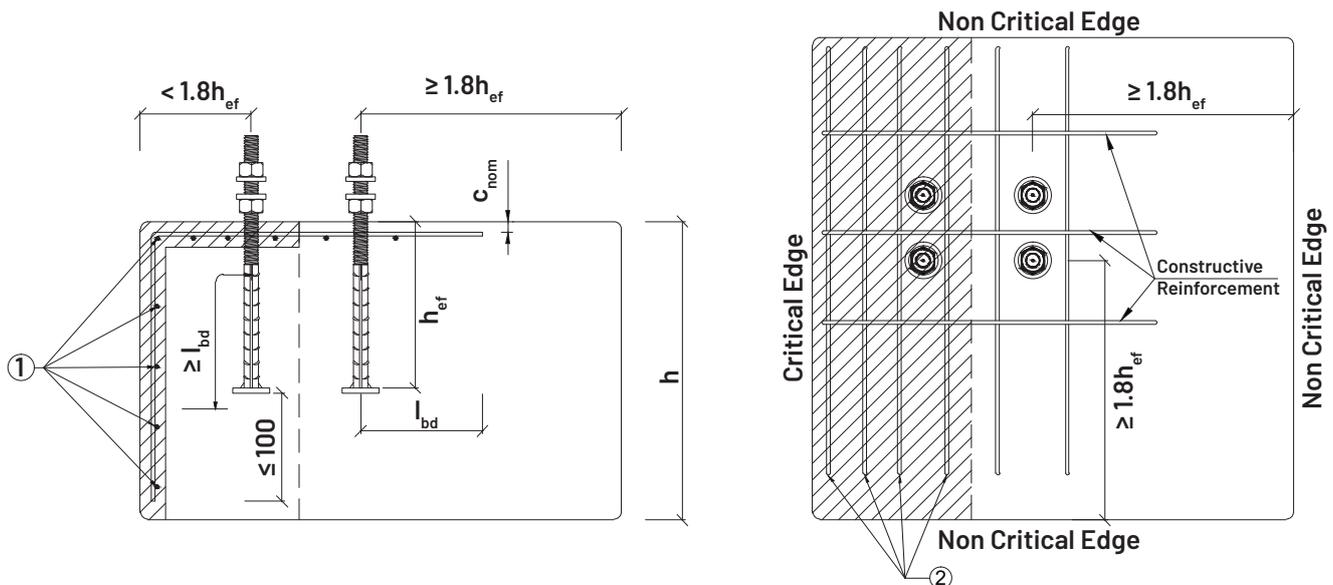
**Table 21. Concrete Splitting Reinforcement for NKP - L Type**
