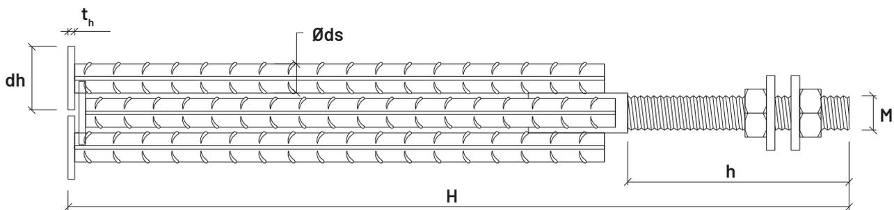
Table 7. SKP - P Type High Capacity Anchor Bolt
