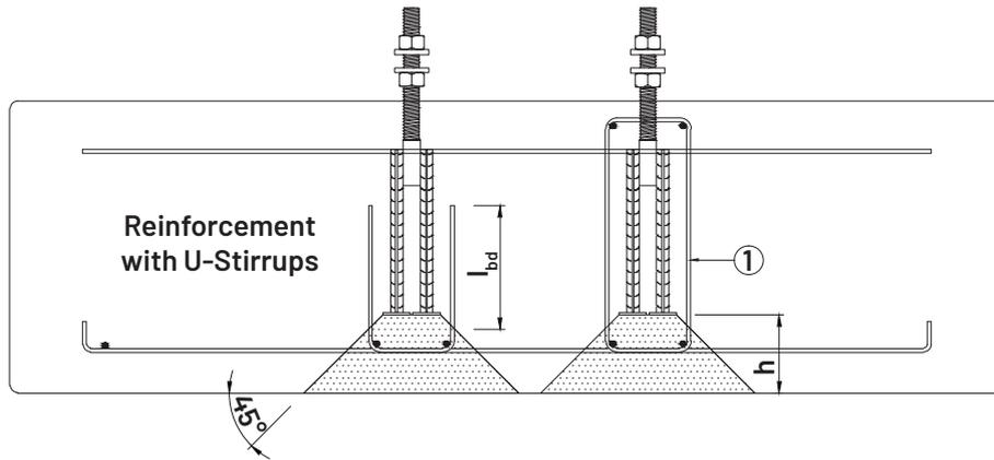
Table 28. Concrete Edge Reinforcement for SKP - L Type High Capacity Anchor Bolt
