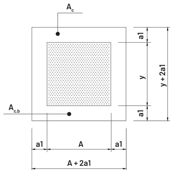
Required splitting reinforcement area
