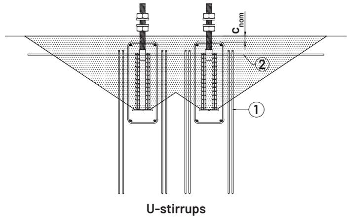
Table 24. Concrete Cone Reinforcement for SKP - L Type High Capacity Anchor Bolt
