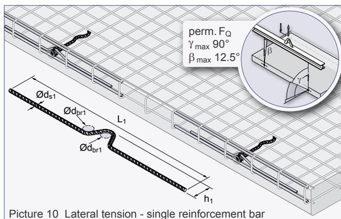
Picture 10 Lateral tension - single reinforcement bar
