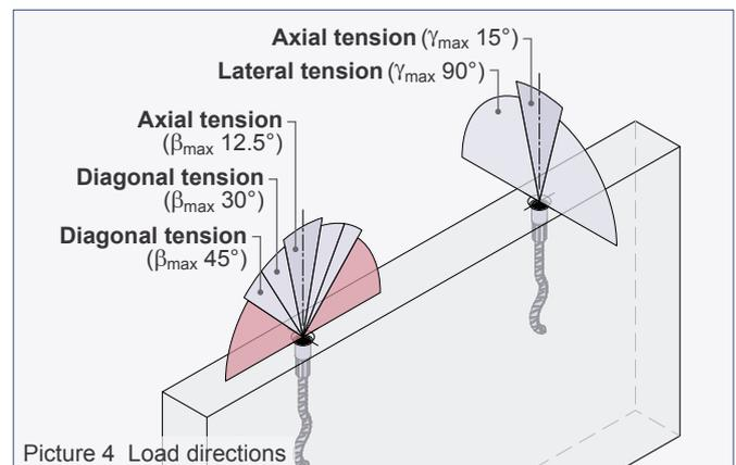
On lateral tension the Threaded transport anchors have only half of the capacity compared to axial loading. However, this is not a limitation as during tilt-up only half of the weight has to be lifted (please refer to the General Installation Instruction).
