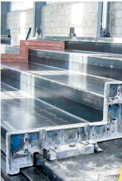
SPB for fixing staircase moulds
