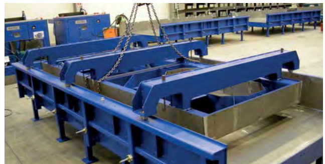
Special shuttering for track roller boxes
