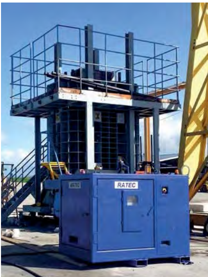
UPP 100 with support shuttering
