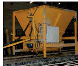
Crane-mounted concrete spreader
