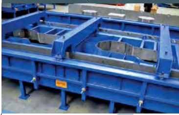
Switzerland Special shuttering
