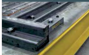
Australia SAS tower special shuttering
