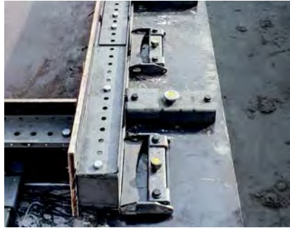
Easy Form with HT stop adapter
