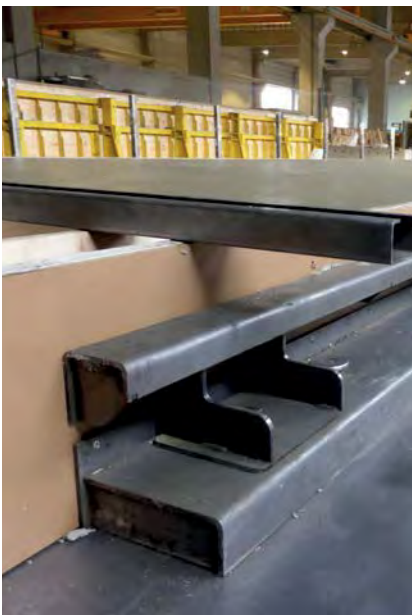
MHS as transversal shuttering
