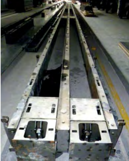
Pile shuttering based on the SAS-MF
