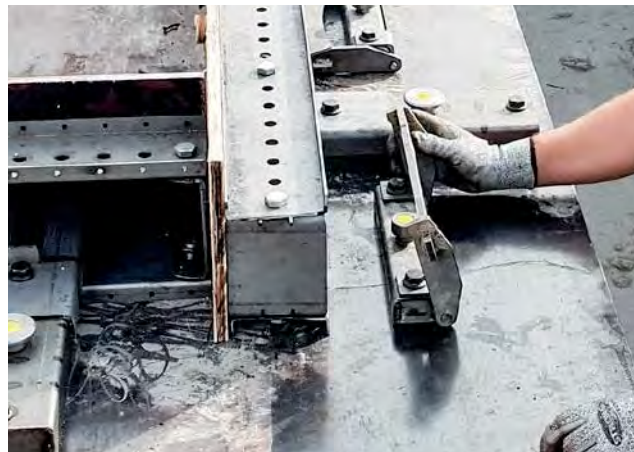
SPB with HT stop adapter and Easy Form (from page 34)
