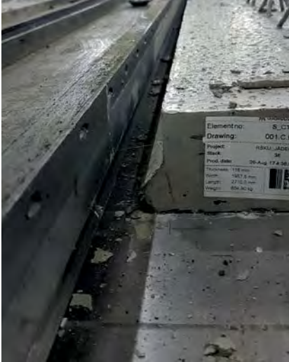
SAS with special profiling of the frontshell
