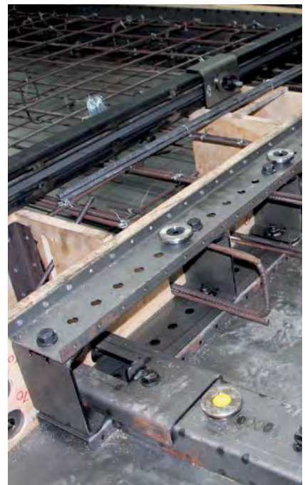
Easy Form with continuous reinforcement
