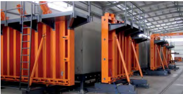
Room module shuttering
