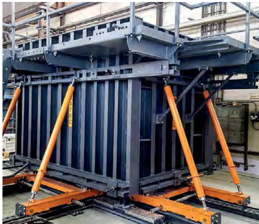
Example: Shuttering for the production of transformer stations measuring 2.4x2.1x2.3 m and 2.9x2.1x2.3 m
