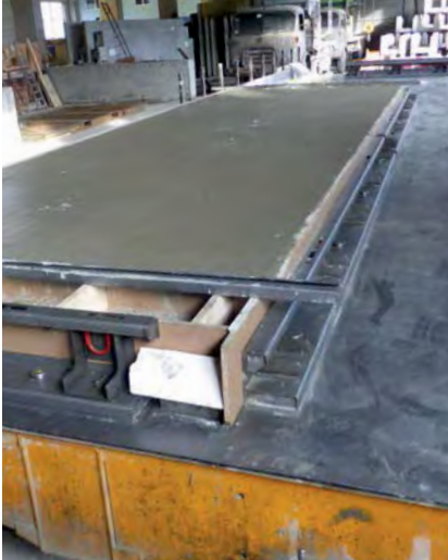
MHS as transversal shuttering
