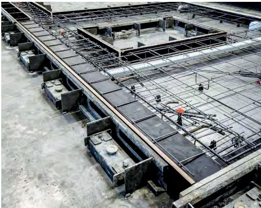
MST as a complete system for external shuttering and recess
