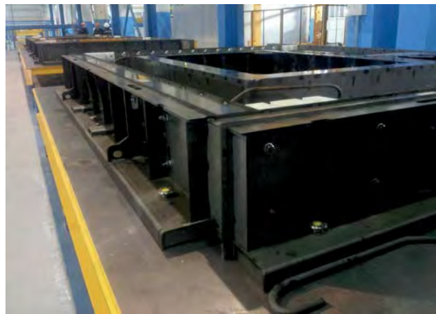
SAS-MF in solid wall production
