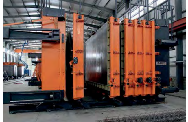
Modular side formwork
